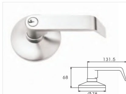
Model: DK-006P/S Clutch function Material for Zinc Alloy or Stainless steel 304 3 brass keys and brass cylinder Schlage cylinder and keys Door width 50MM in normal Finish: US26D or Stainless steel
